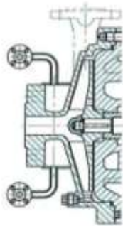
Heat keeping jacket in casing
